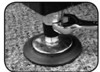
Tighten Locking Nut
